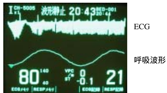
Fig.1. Noise by EMI between cellular phone and ECG monitor
